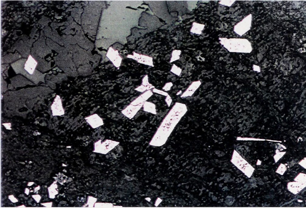
Fig.27: Photomicrograph of euhedral arsenopyrite crystals in quartz and surrounding wall rock. Reflected light on polished surface, crossed-polars. Bottom edge of picture is 2.8 mm in length.
